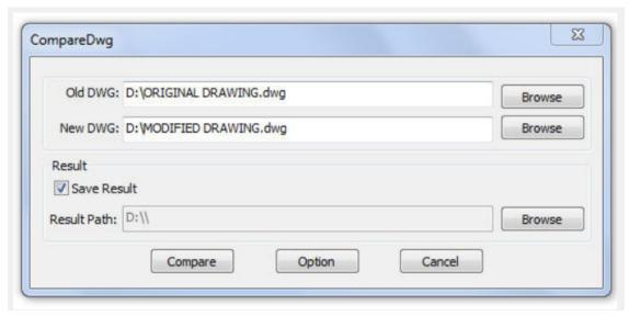
In this window, you have to browse the old DWG (original drawing) and the new DWG (drawing modified). You can also assign a path to save the compared drawing. Then select the button Option to setup the comparison parameters.
