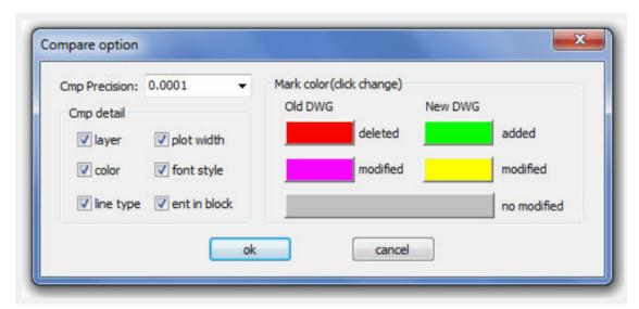
After setting up the comparison parameters such as: colors, layers, line type, etc. select Ok to confirm these parameters. Note: Pay attention to the mark color because the deleted, modified and added objects will assume these into the compared drawing. Then select the button Compare in the window below to compare both drawings.
