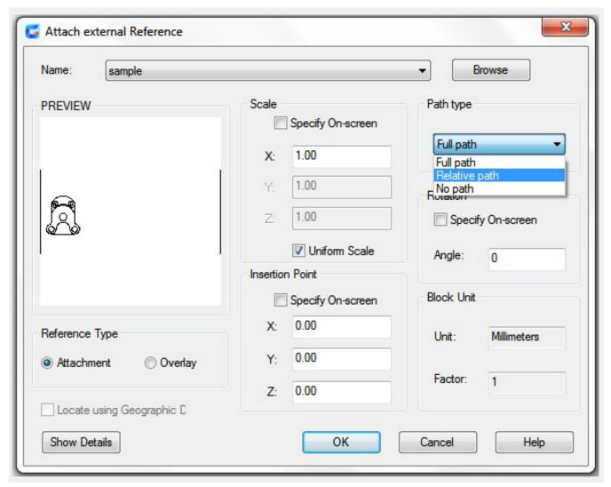
When you attach an external reference, its elements like layers (XREF), linetypes (LINETYPE), text styles and other elements are not added to the current drawing, but also linked from the referenced file.
