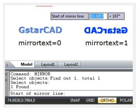
Text created with the <u>TEXT</u>, <u>ATTDEF</u> or <u>MTEXT</u> commands, attribute definitions and variable attributes will be affected by MIRRTEXT. Regardless of MIRRTEXT setting, the text and constant attributes that are part of an inserted block are reversed when the block is mirrored
