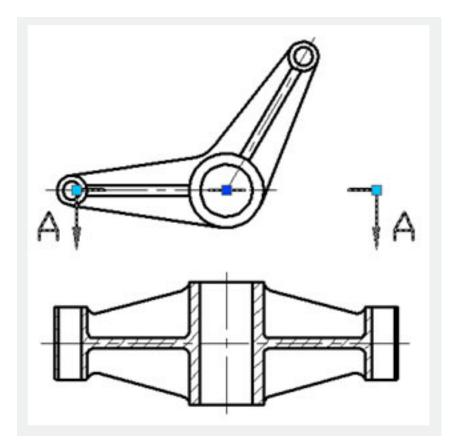
Drag the grip of the dynamic block, the section symbol can be stretched outward and rotated around the center, and you finish the section symbol mark as below:
