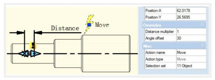
Select the Dynamic Block and then move the right side grip. You will find it can only move in the direction of  $30^{\circ}$  as it is shown in the follow picture. The direction of action can change according to the Angle Offset.
