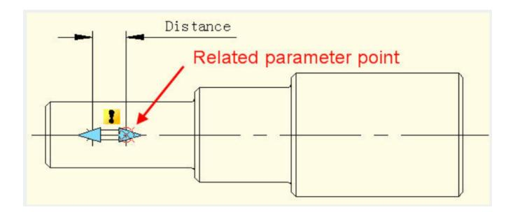
The parameter point we mentioned corresponds to the operate point of Move. After exiting Block Editor you can drag this point to make dynamic block change correspondingly.
