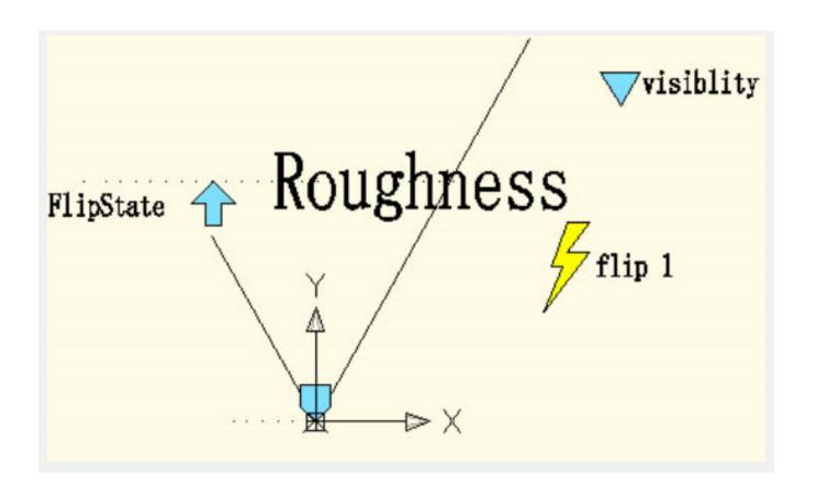
Use the same method to add a pair of flip parameter and action of the vertical direction, as shown in below picture.
