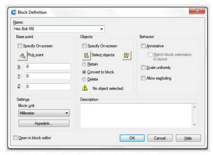
The base point is used as a reference for positioning the block when you insert it.
