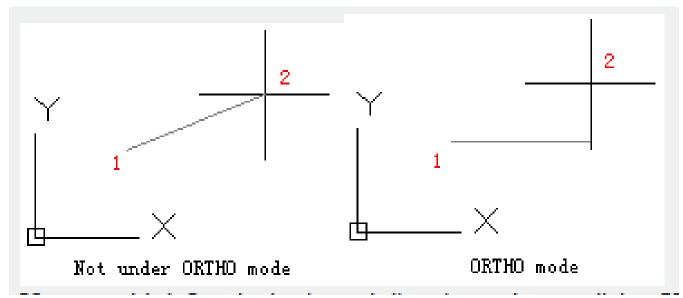
Users could define the horizontal direction to be parallel to X axis of UCS and the vertical direction to be parallel to Y axis of UCS. In 3D viewport, the ORTHO is defined to be parallel to Z axis of UCS. The command prompt displays +Z or -Z according to angle of Z axis.
