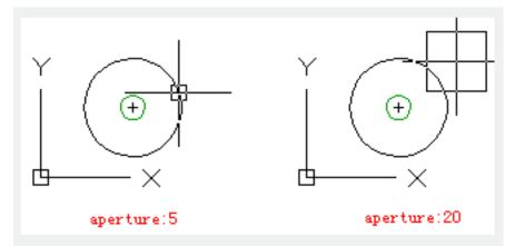
The APERTURE command could control object Aperture box rather than Pick box that displayed under the command prompt of "select object".
