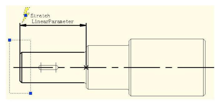
Because the follow-up operation will not stretch step shaft by grips of this linear parameter, the grip's number of linear parameters can be modified as "0".
