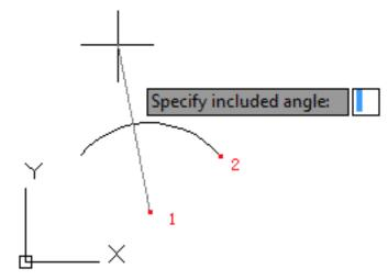
• Chord length: The point 1 is center of arc. The chord length is the distance from the point 2 to the endpoint. Users could create a major arc or minor arc by specied chord length. If inputting a positive chord length value, it will create a minor arc in anticlockwise; if inputting a negative chord length value, it will create a major arc in anticlockwise.
