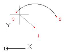
• Angle: The point 1 is center of arc. The included angle is from the point 2. It is created in anticlockwise. If inputting a negative angle, the arc will be created in clockwise direction.
