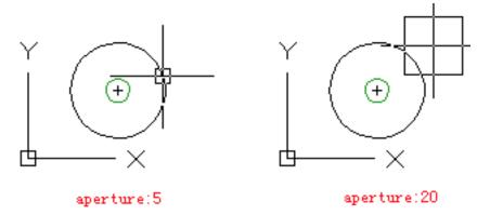
The APERTURE command could control object Aperture box rather than Pick box that displayed under the command prompt of "select object".
