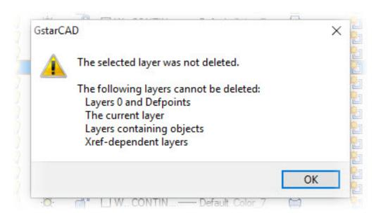
The solution is by using LAYDEL command,
