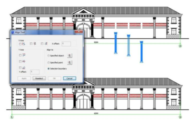
As an example, we will put this tool in action. We can apply this tool to align a high quantity of objects (columns) in the correct place in this complex drawing as shown in the picture below:
