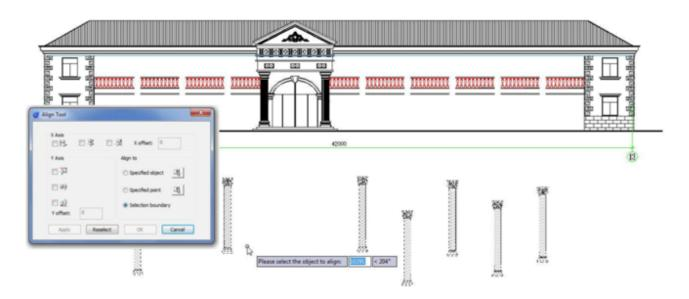
After you have selected the objects, the Align tool settings window will pop up: first we have to check the option Top object under Y axis alignment. After check this option the objects (columns) will be aligned at same level:
