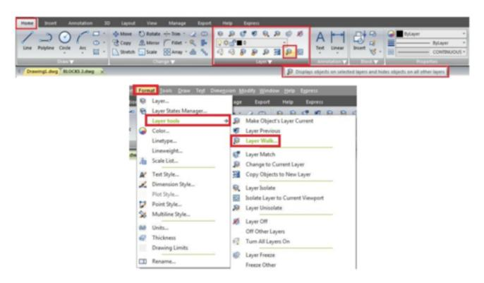
With this tool, you can quickly check if your objects are placed correctly in their layer. You can turn off restore on exit if you find the one placed in wrong layer and move it.
