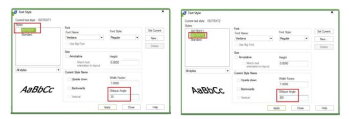
Now try to create text (single or multi line) with different styles and angle combination, then change the rotation to 30 deg or -30 deg. It depends on where you want to put it. See next image as reference.
