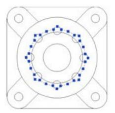
4.Start again the boolean operations, select option "subtraction" and check "Delete the entity choosen by second selection", as shown.
